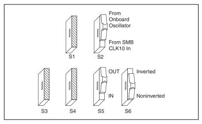
Figure C-6. Drive Noninverted External CLK SMB
